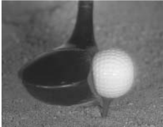
FIGURE 5.24 During its contact with a golf club, a golf ball is distorted. As the ball moves away from the club, and while the ball recovers its normal spherical shape, its elastic potential energy is transformed into (additional) kinetic energy.
