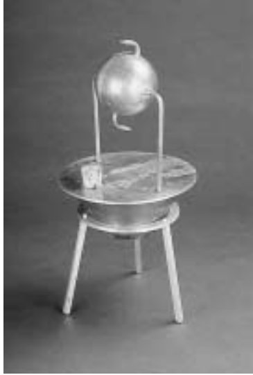
FIGURE 6.6 A model of Heron's aeolipile. Steam produced in the boiler escapes through the nozzles on the sphere, causing the sphere to rotate.
