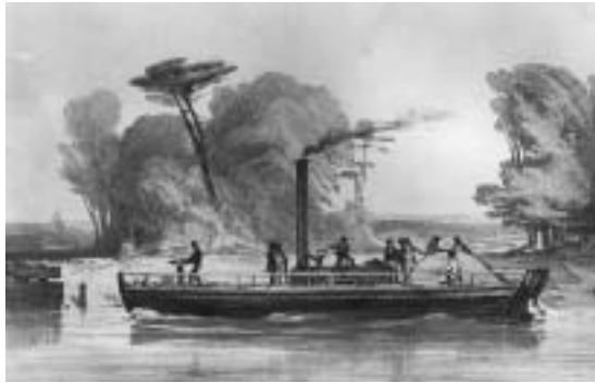
FIGURE 6.11 The Charlotte Dundas , the first practical steamboat, built by William Symington, an engineer who had patented his own improved steam engine. It was tried out on the Forth and Clyde Canal in 1801.
