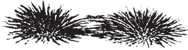
FIGURE 10.21 Needle-like iron oxide crystals in the magnetic field of a bar magnet. The bar magnet is under a paper on which the iron oxide crystals have been spread.
