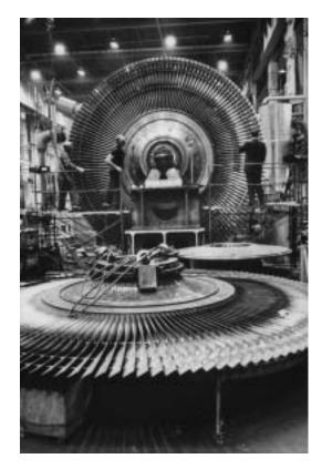
FIGURE 11.10 Steam turbine rotors.
