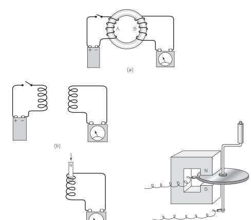
FIGURE 11.3 Various ways of producing electromagnetic induction.
